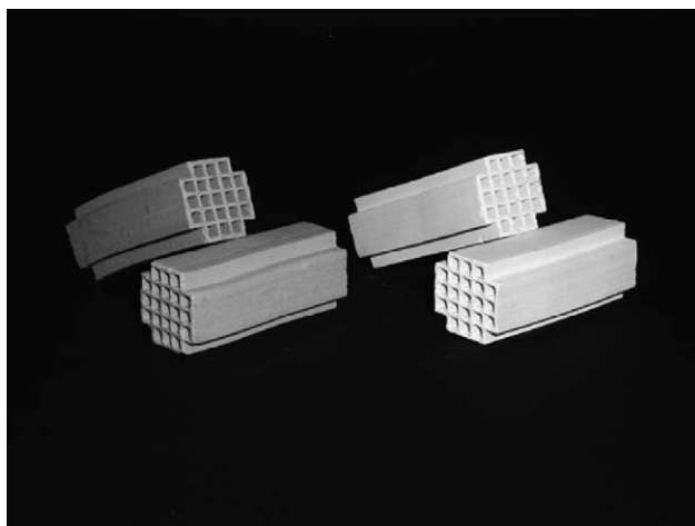
Fig. 2. Photograph of 21 cell monolithic supports prepared with a 10 wt.% of PGA before (left) and after (right) the heat-treatment process (550 °C for 4 h).
